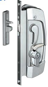
**Operation:** A reliable all-metal mortise lock for sliding doors having a latch bolt that is retracted by operation of either an outside or inside lever. Once latched it may be locked (or unlocked) from either side by key.
