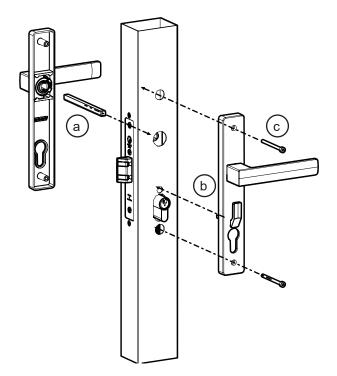
\*\* Note if using the Austral Mortise lock; please use the spindle supplied with the mortise lock.
