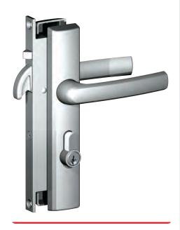
**Operation:** A reliable mortise lock for hinged security doors having a pivoting latch bolt that is retracted by operation of either an outside or inside lever. Closing the door causes an auxiliary bolt to release the latch bolt enabling it to enter the strike plate. Once fully extended it may be locked (or unlocked) from either side by key.
