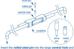
tap with hammer until it is fully inside the *coupling*.
