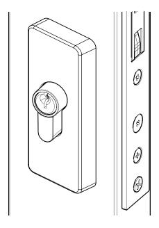
Use a screw driver to push the escutcheon down to release it from the bottom of the base
